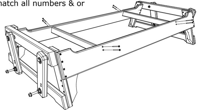
3. Attach (D) Bearing Arm Supports to Glider Base using 4 - 2 1/2" Screws per side, be sure to match all numbers & or letters.
