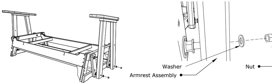
5. Attach (B) Back Assembly to (A) Seat Assembly using 6 - 2" Wafer Bolts, be sure to Match all numbers & or letters, tighten Wafer Bolts with included Hex Key.
