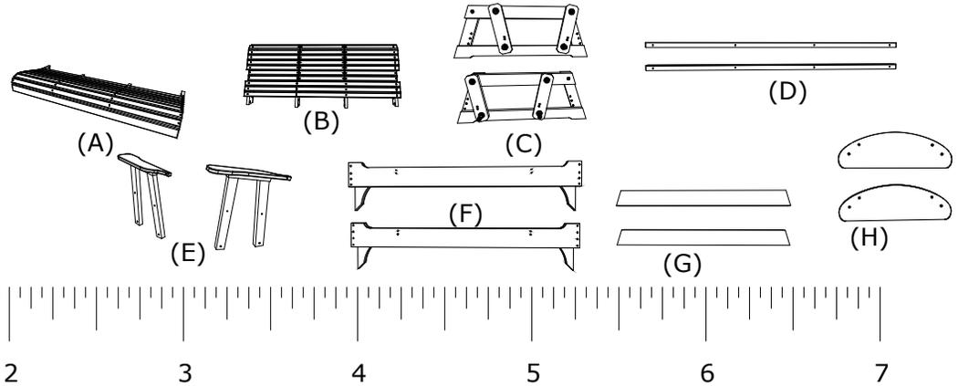
1. Attach (F) Front-Back Crosspieces to (C) Glider Base's Using 14 - 2" Screws per side, be sure to match all numbers & or letters.
