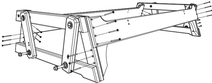
2. Attach (G) Crosspiece Supports to Front-Back Crosspieces using 4 - 2" Screws per side, be sure to match all numbers & or letters.
